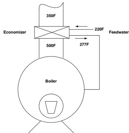
Hot flue gas contains a lot of wasted energy and it is very beneficial to put this energy back into the boiler with heat recovery equipment. The rule of thumb for reducing stack temperature is: for every 40 degrees F the temperature is reduced, a 1% efficiency increase occurs. In this case lowering stack temperature 150 degrees F will result in an efficiency increase of approximately 3.75%.
